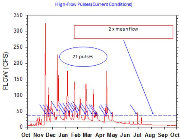
**Figure 3. Hydrograph Displaying High-Flow Pulses with Developed Use/Land Cover**
