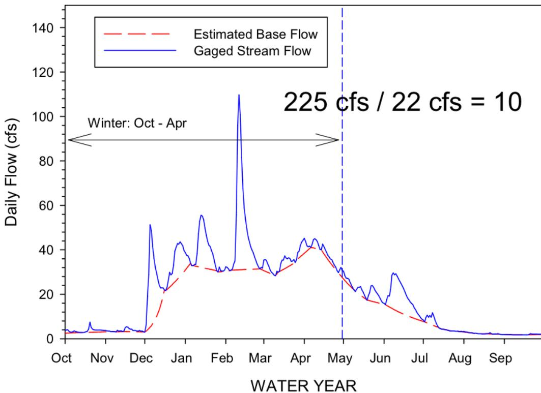
**Figure 5. Hydrograph Illustrating Determination of 2-Year Peak:Mean Winter Base Flow Ratio (note: 2-year frequency peak flow rate did not occur in the year portrayed)**
