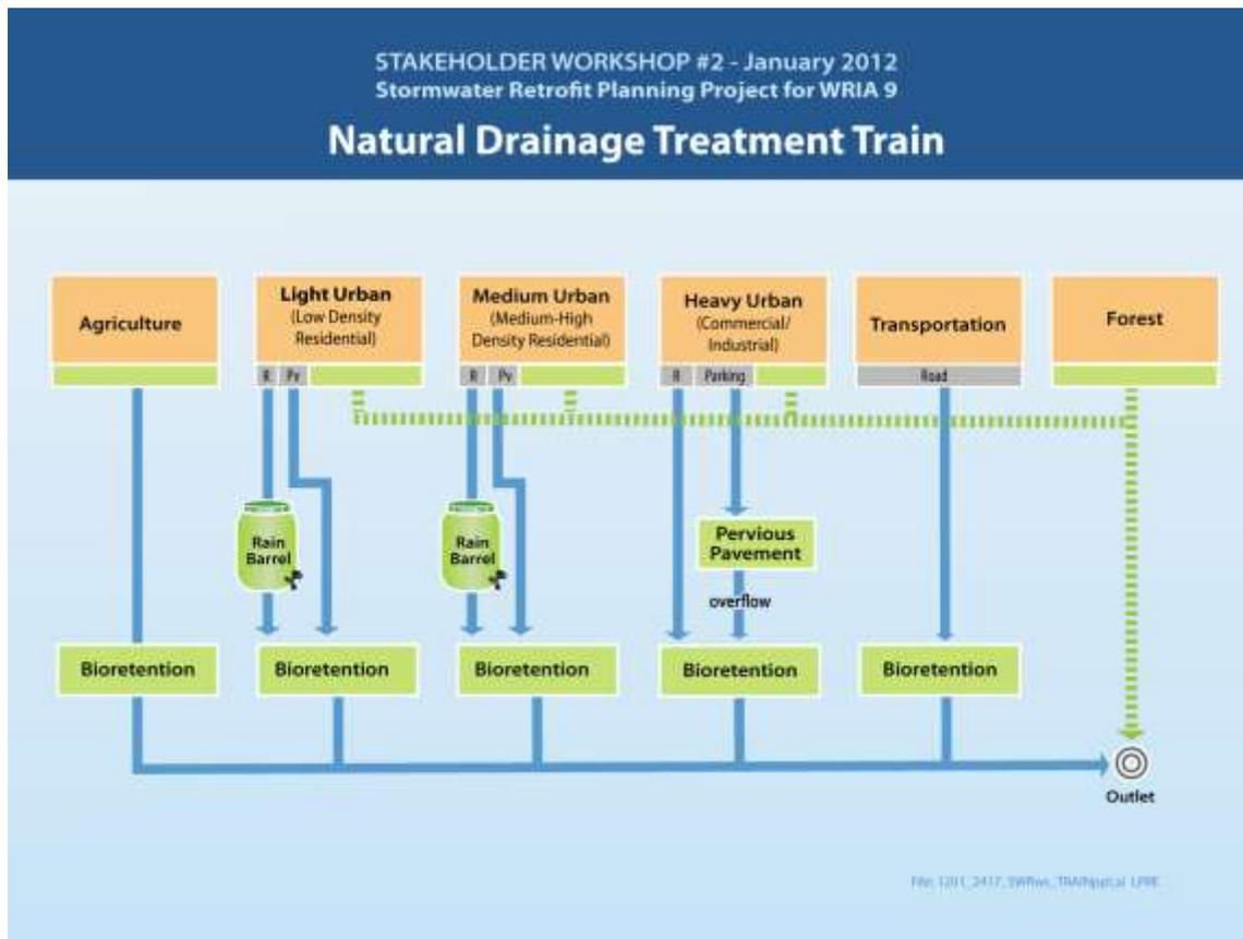
Figure 1. Natural Drainage Treatment Train
