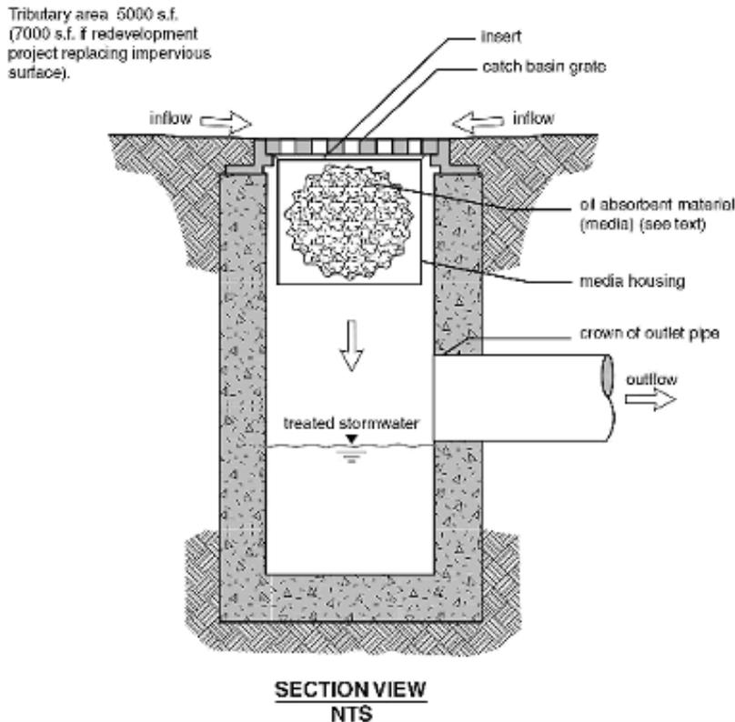
The typical design of a catch basin insert is a set of filters that are specifically chosen to address the pollutants expected at that site (Source: King County, Washington, 2000)
