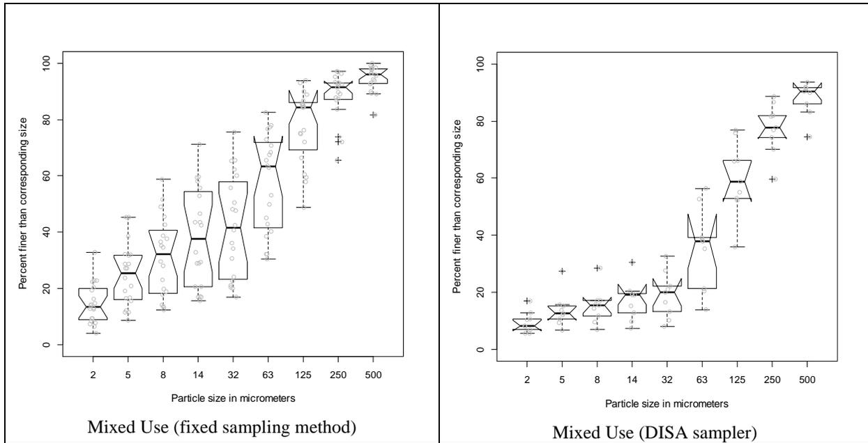
Figure 10. Fixed point and DISA sampling from the same land use; different monitoring periods
