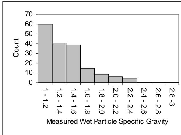
Figure 4. Particle specific gravity distribution
