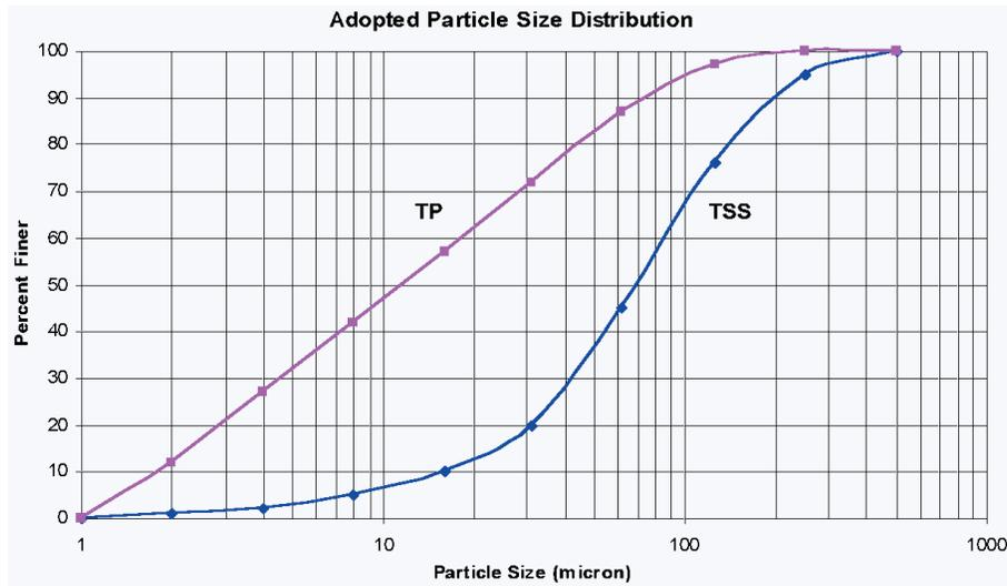
Figure 16. Possible PSD for Melbourne and Brisbane fully developed catchments.
