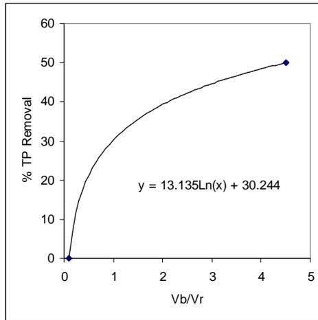
Figure 15. Total phosphorus removal as a function of  $V_b/V_r$
