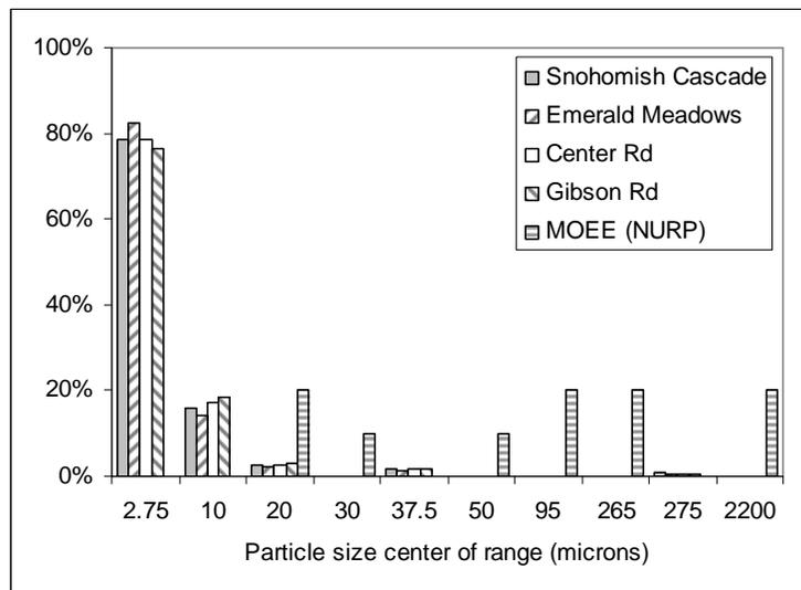
Figure 7. Particle size distributions<sup>†</sup> comparing four regional sites to the NURP data as given in MOEE (1984)
