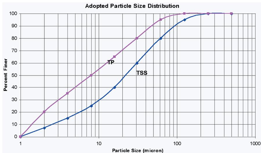
Figure 17. Possible PSD for developing catchments in Melbourne and Brisbane.
