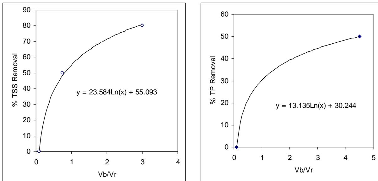
Figure 19. Percent TSS and TP Removal as a function of  $V_b/V_r$
