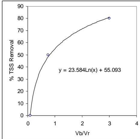
Figure 13. Percent TSS Removal as a function of  $V_b/V_r$
