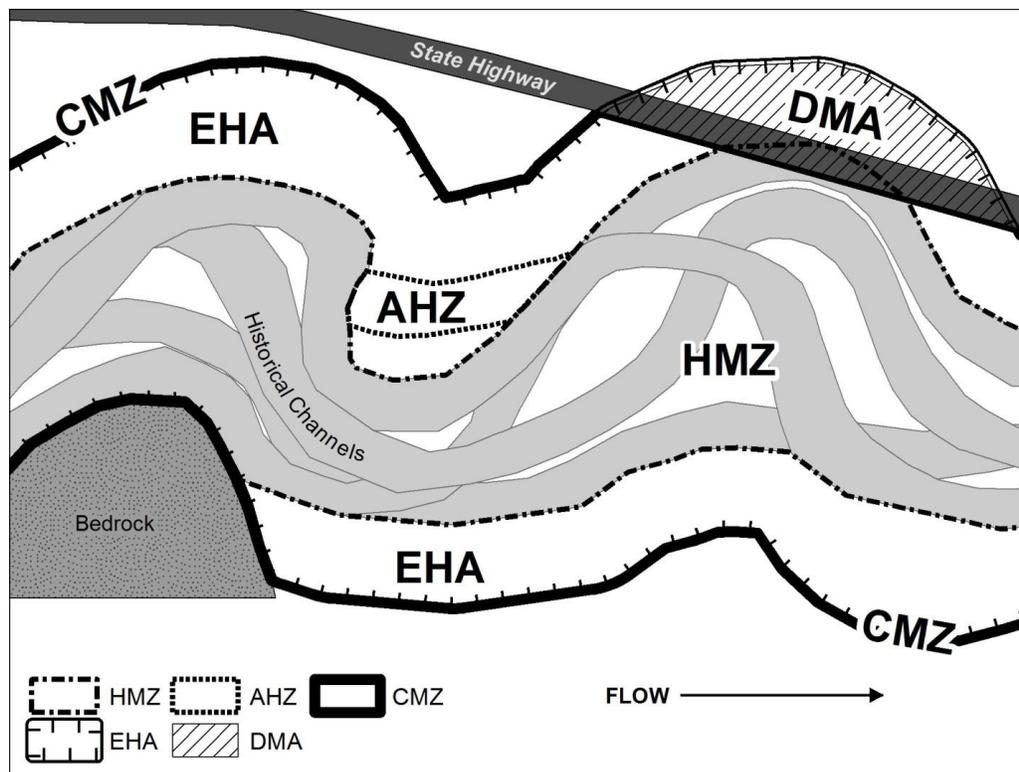
**Figure A-1. Planview schematic of the Channel Migration Zone (CMZ) as the combination of the Historic Migration Zone (HMZ) plus the Avulsion Hazard Zone (AHZ) plus the Erosion Hazard Area (EHA) minus the Disconnected Migration Area (DMA). Modified from Rapp and Abbe (2003).**
