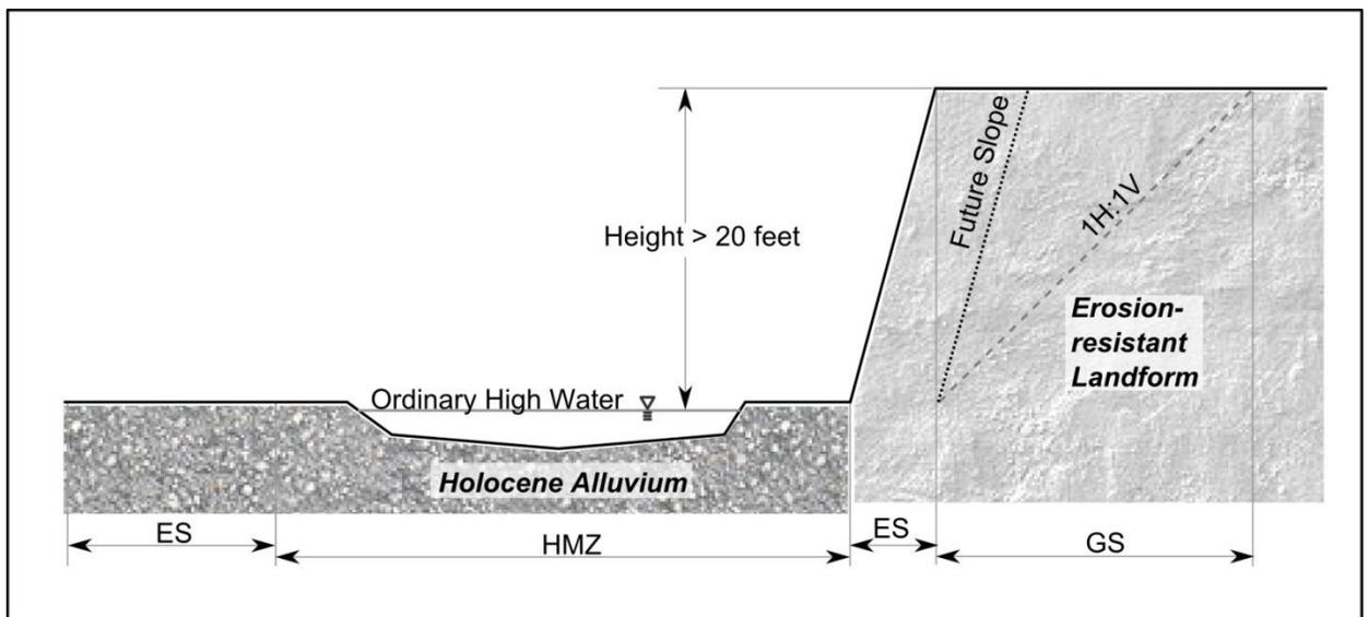
**Figure A-3. Cross-section schematic of Erosion Hazard Area/ Geotechnical Setback illustrating that a Geotechnical Setback (GS) should be measured at a 1Horizontal:1Vertical (1H:1V) slope at the outer edge of the Erosion Setback (ES), as described in section IV.E.1.a. The narrower ES on the right side of the Historical Migration Zone (HMZ) illustrates an ES calculated using a lower channel migration rate in an erosion resistant landform, as described in section IV.D.1.d.**
