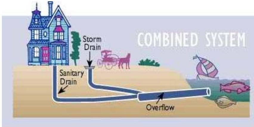
**Fig. 1 – Illustration of an older combined system (pre-1950's) in which sanitary sewage is conveyed in one pipe and stormwater sewage conveyed in another.**
