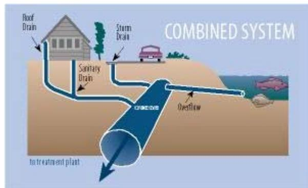
**Fig. 3 – Illustration of a typical modern combined sewer system (post-1950's).**
