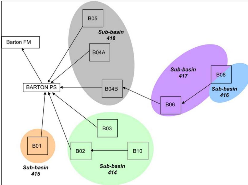
**Figure 4.1 Barton CSO Basin Flow Meter Schematic**
