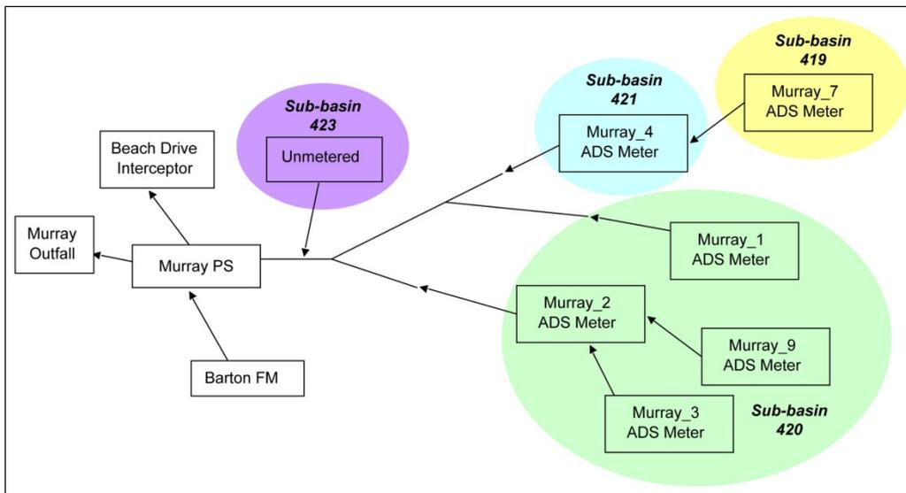
**Figure 4.2 Murray CSO Basin Flow Meter Schematic**
