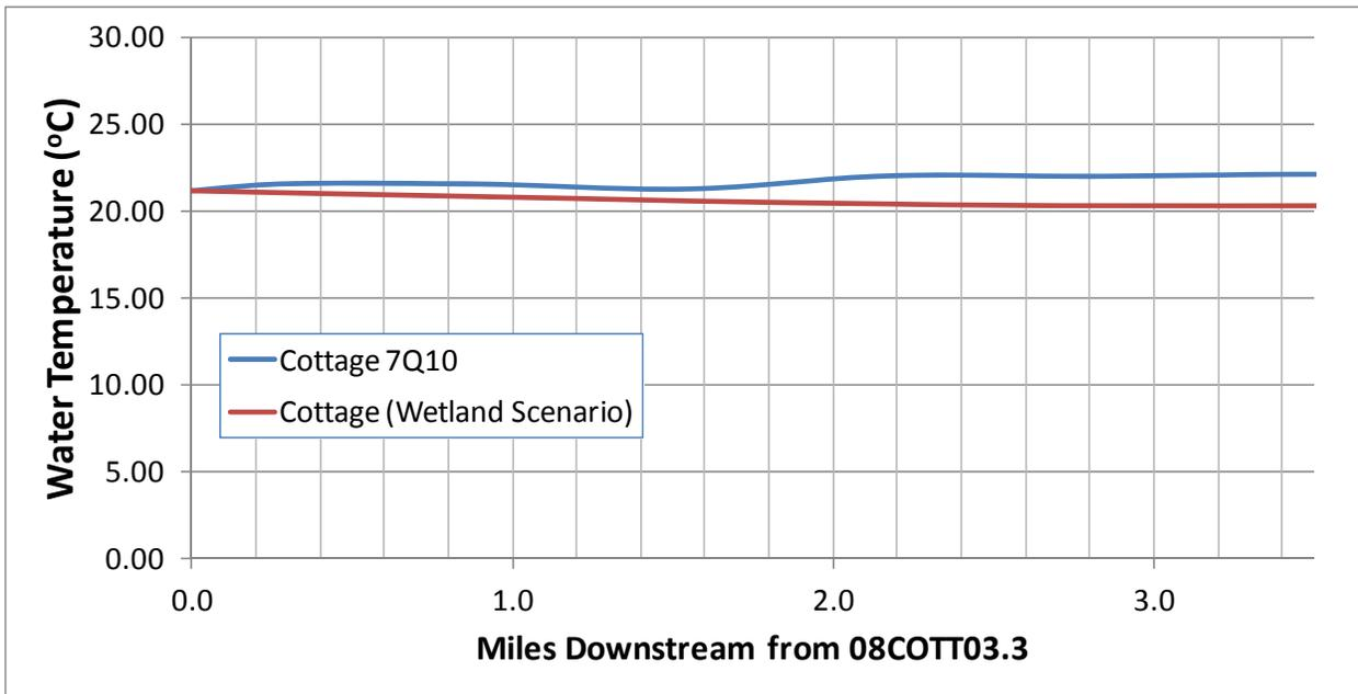
**Figure 4-3. Comparison of the effect of an increase of 8.8 cfs at the upstream boundary (below Cottage Lake) of the Ecology Current Critical Conditions (7Q10) QUAL2Kw model of Cottage Lake Creek on summer maximum stream temperature**
