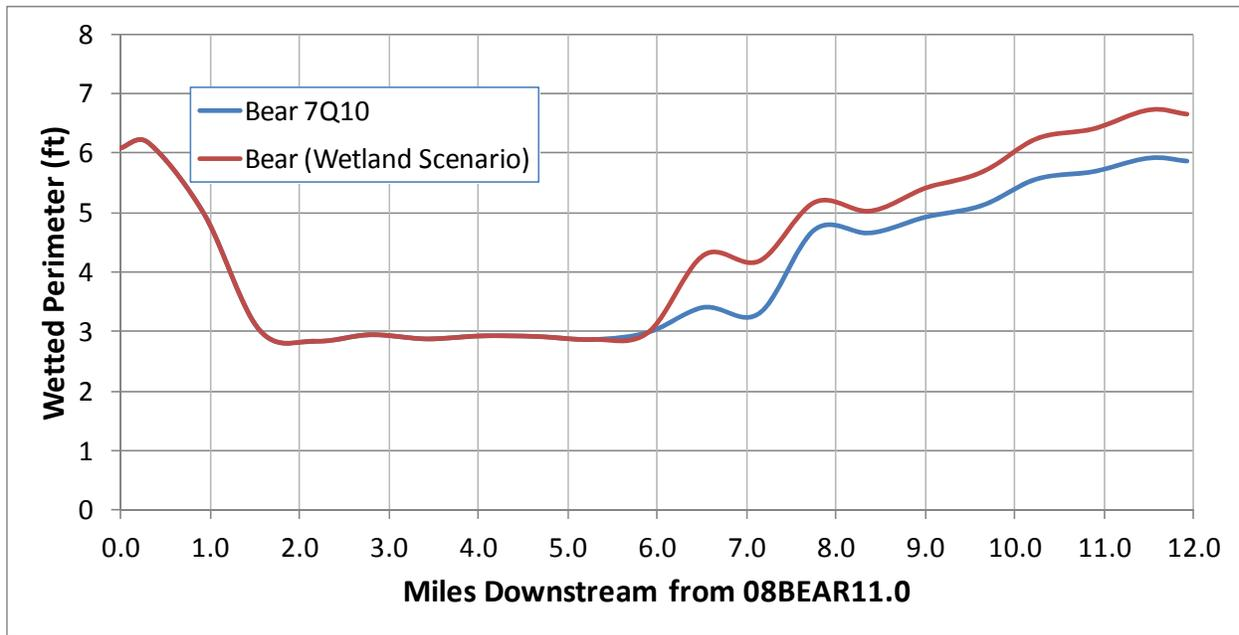
**Figure 4-8. Comparison of the effect of an increase of 8.8 cfs at the upstream boundary (below Cottage Lake) of the Ecology Current Critical Conditions (7Q10) QUAL2Kw model of Bear Creek on wetted stream perimeter**
