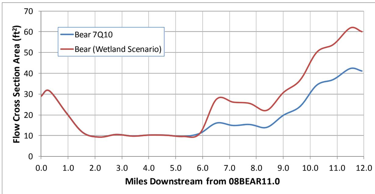
Figure 4-6. Comparison of the effect of an increase of 8.8 cfs at the upstream boundary (below Cottage Lake) of the Ecology Current Critical Conditions (7Q10) QUAL2Kw model of Bear Creek on wetted stream cross-sectional area
