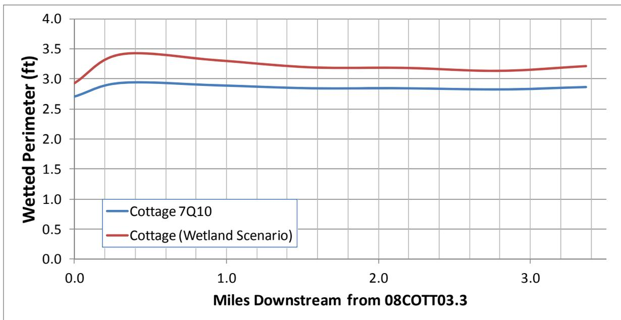
Figure 4-7. Comparison of the effect of an increase of 8.8 cfs at the upstream boundary (below Cottage Lake) of the Ecology Current Critical Conditions (7Q10) QUAL2Kw model of Cottage Lake Creek on wetted stream perimeter
