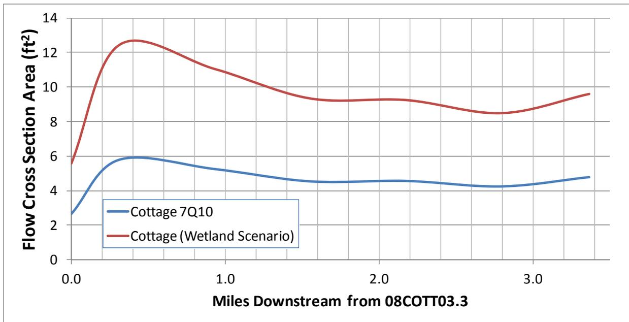
**Figure 4-5. Comparison of the effect of an increase of 8.8 cfs at the upstream boundary (below Cottage Lake) of the Ecology Current Critical Conditions (7Q10) QUAL2Kw model of Cottage Lake Creek on wetted stream cross-sectional area**
