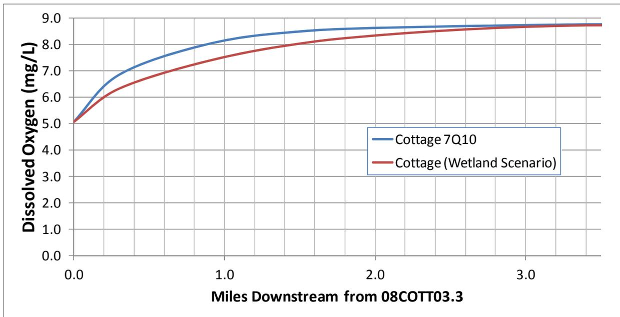
**Figure 4-1. Comparison of the effect of an increase of 8.8 cfs at the upstream boundary (below Cottage Lake) of the Ecology Current Critical Conditions (7Q10) QUAL2Kw model of Cottage Lake Creek on summer minimum dissolved oxygen concentrations**
