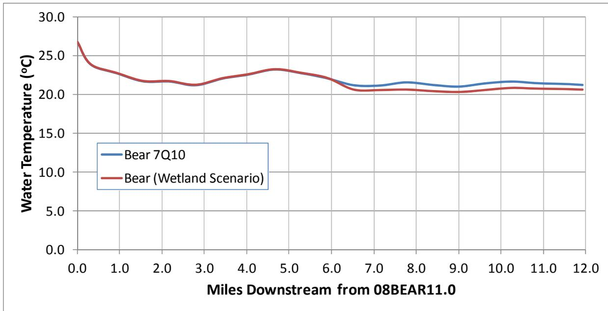
**Figure 4-4. Comparison of the effect of an increase of 8.8 cfs at the upstream boundary (below Cottage Lake) of the Ecology Current Critical Conditions (7Q10) QUAL2Kw model of Bear Creek on summer maximum stream temperature**
