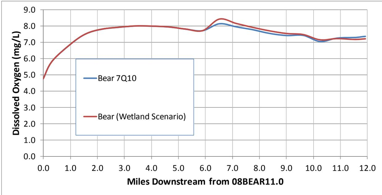
**Figure 4-2. Comparison of the effect of an increase of 8.8 cfs at the upstream boundary (below Cottage Lake) of the Ecology Current Critical Conditions (7Q10) QUAL2Kw model of Bear Creek on summer minimum dissolved oxygen concentrations**
