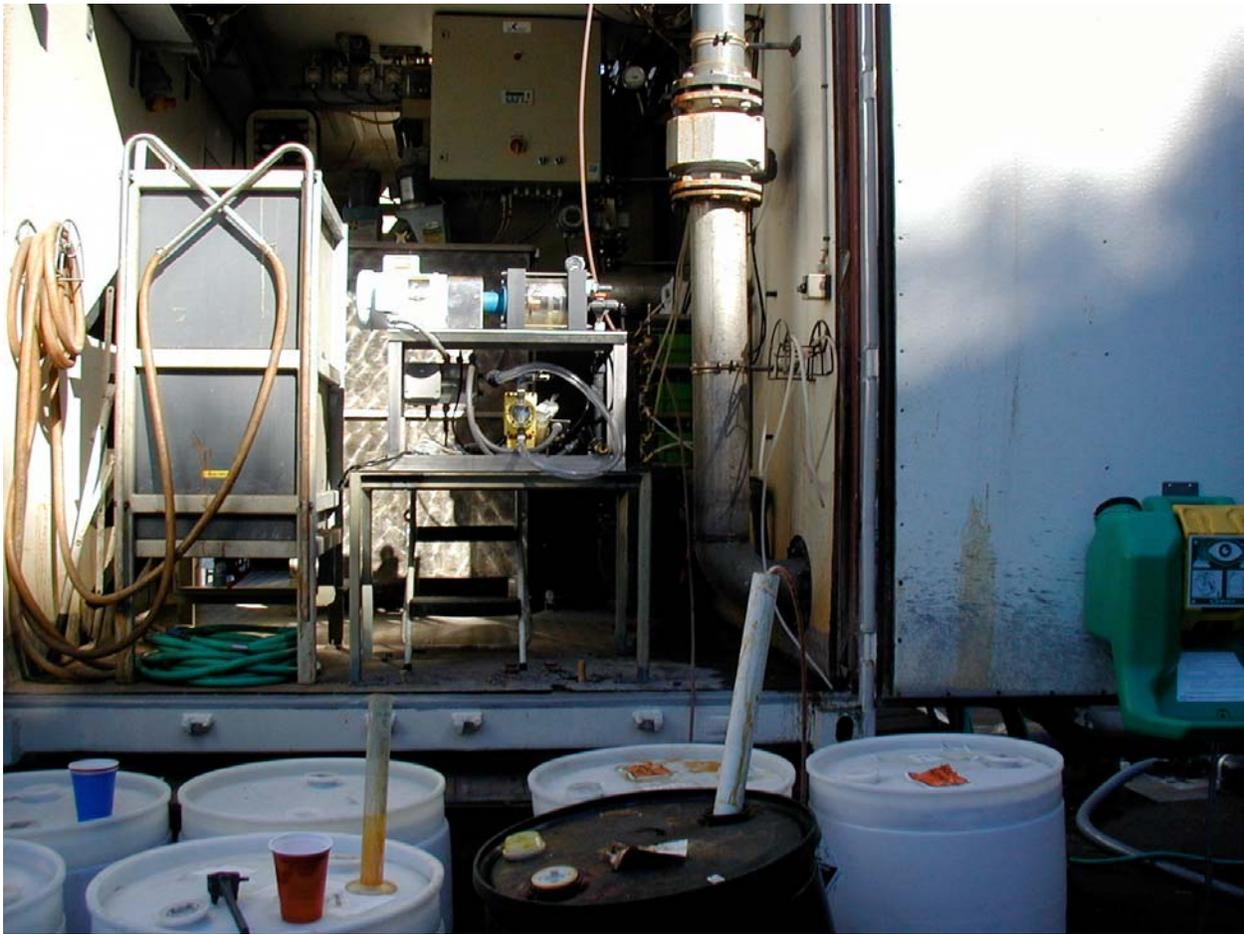
*Figure 3. USFilter/Kruger Pilot Unit, Back End of Trailer - Coagulant and Polymer Feed Equipment*
