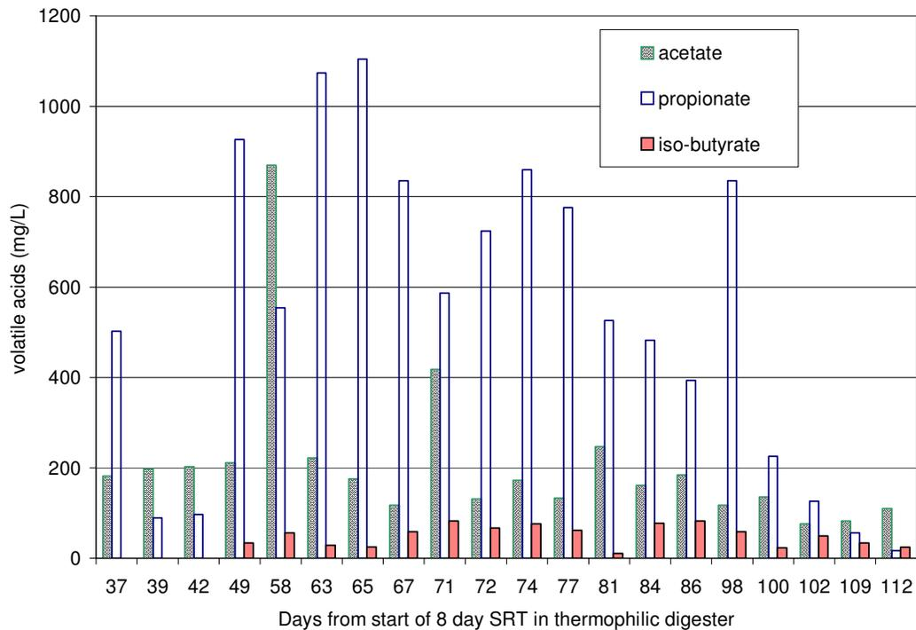
Figure 4. Volatile fatty acid concentrations in the thermophilic digester at sample days from start of 8d – 8d SRT operation
