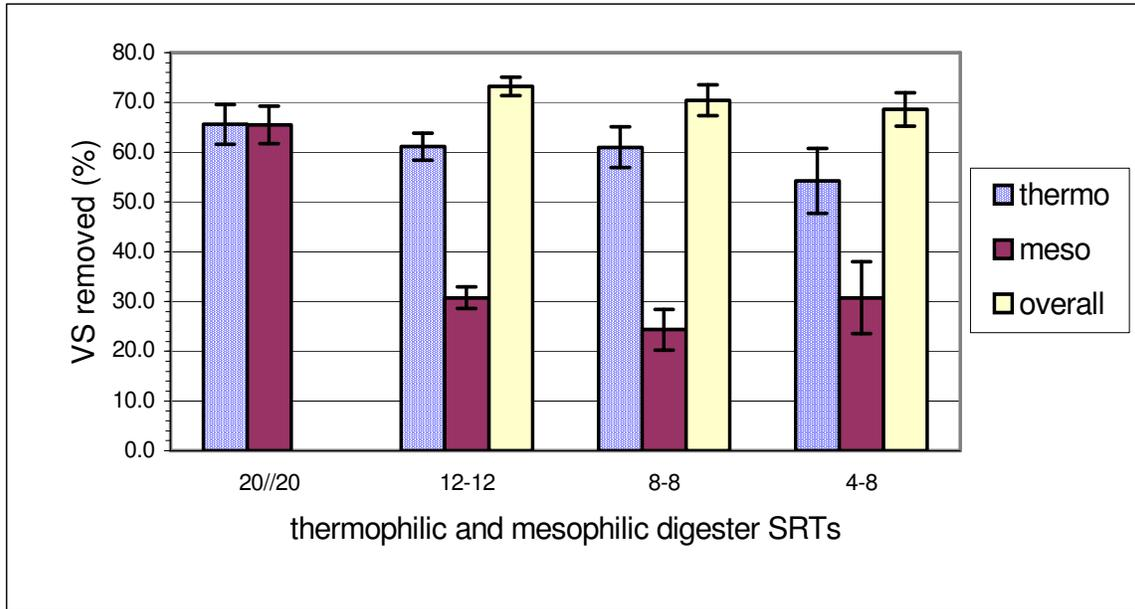
Figure 2. Percent of feed volatile solids destroyed for total system and in thermophilic and mesophilic digesters at each test condition.
