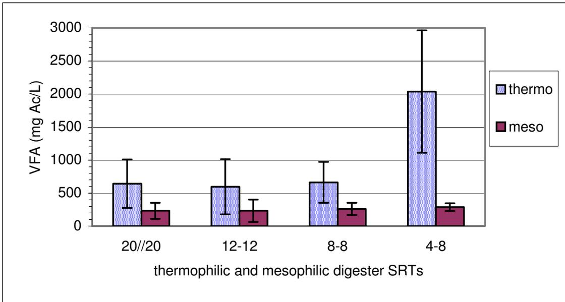
Figure 3. Total volatile fatty acid concentration in thermophilic and mesophilic digesters at each test condition.
