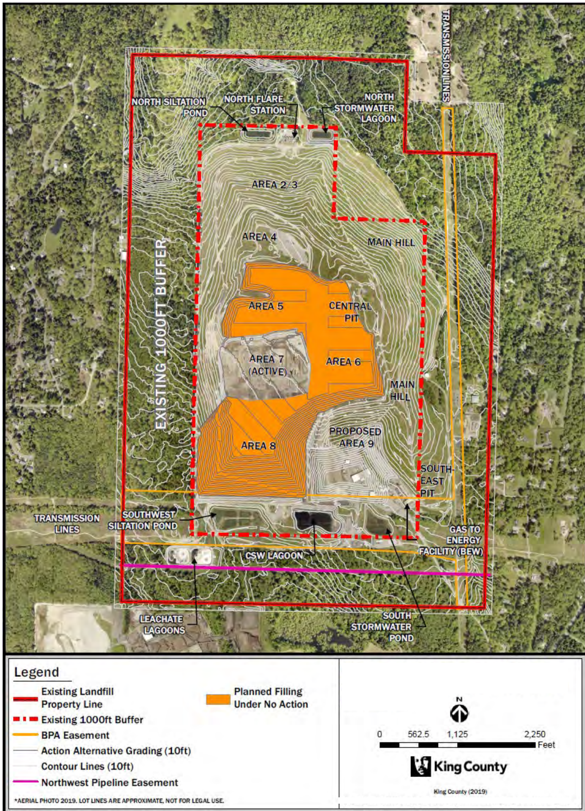
Figure 2. Waste Disposal Areas, Buffer, Easements, and Other Facilities
