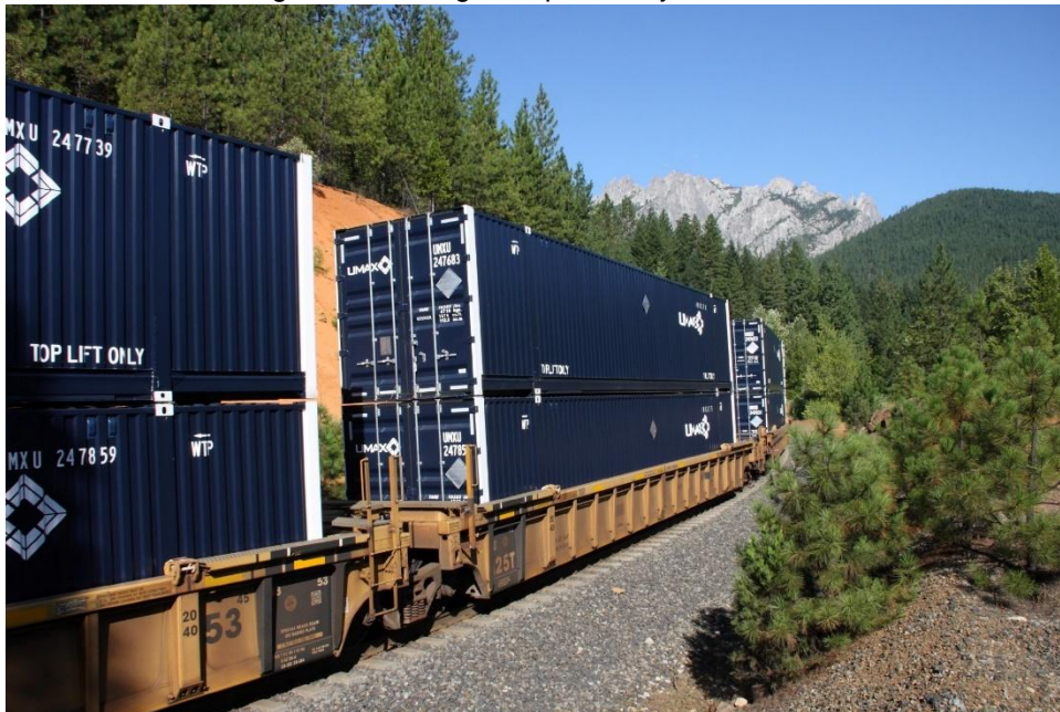
Figure 3-1: Double-Stack Rail Transport is the Standard Configuration for WEBR
