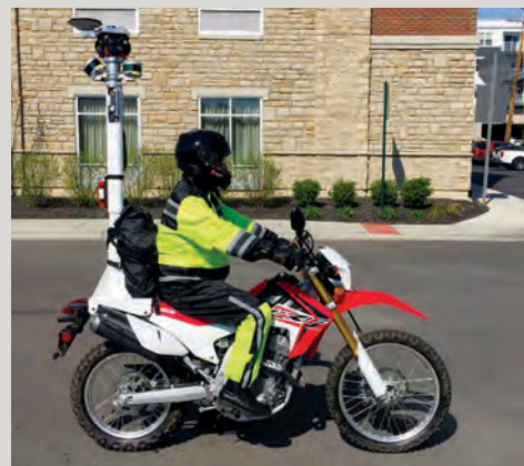
King County Parks employs the use of remote LiDAR (Light Detection and Ranging) to create an inventory of trail surfaces and trailside assets (shown here on the back of a motorcycle).
