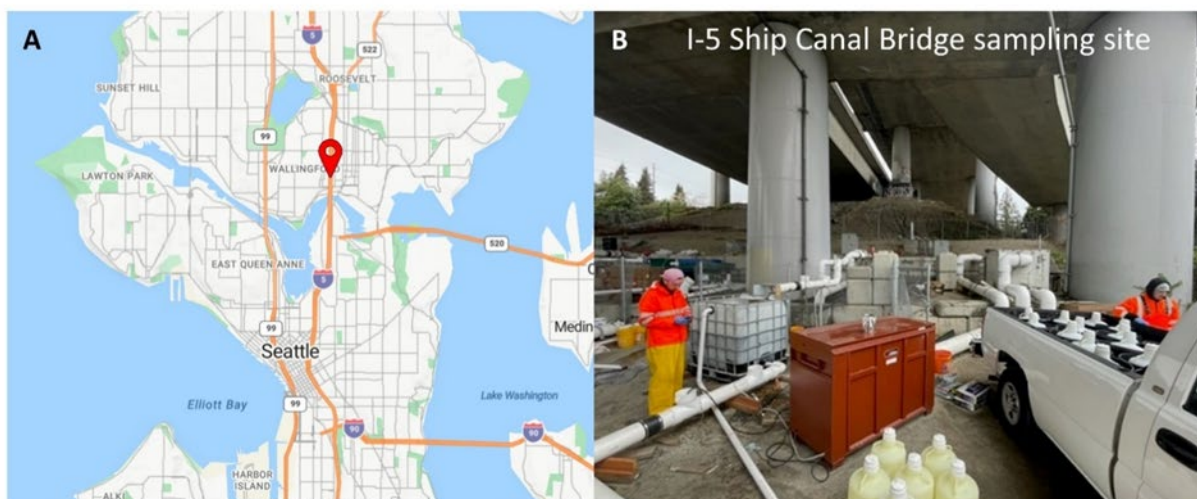
Figure 3. A) Location of the I-5 WSDOT Ship Canal Bridge runoff test site used to collect stormwater for column dosing with sampling. B) King County's Field Science Unit collecting stormwater for column dosing.
