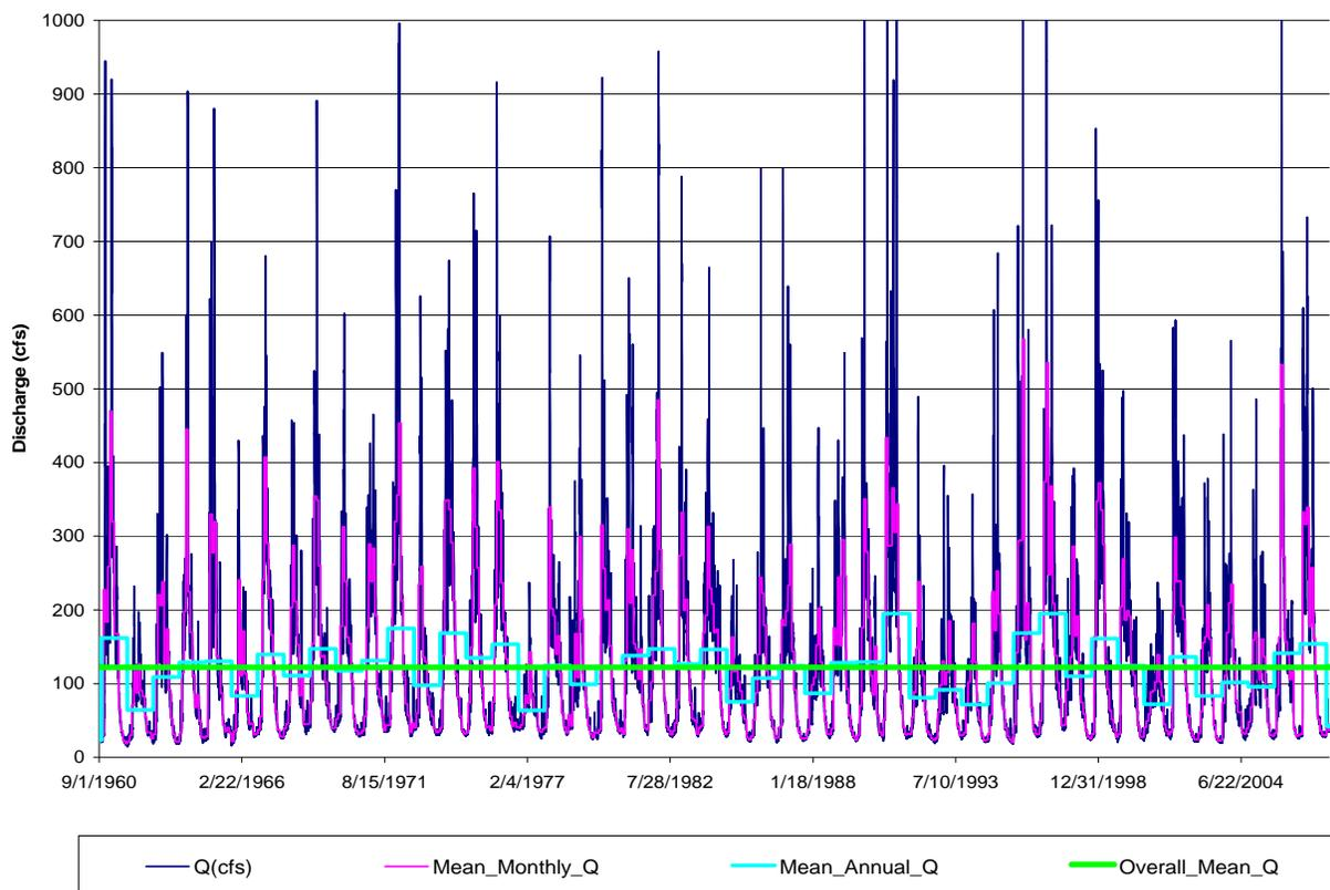
**FIGURE 2.** Historic flow conditions near the mouth of Soos Creek Washington, USGS Gauge 12112600 (1960-2007). Mean daily (dark blue line), mean monthly (pink line) and mean annual (light blue line), and overall mean discharge (light green line) values are represented in the graph.
