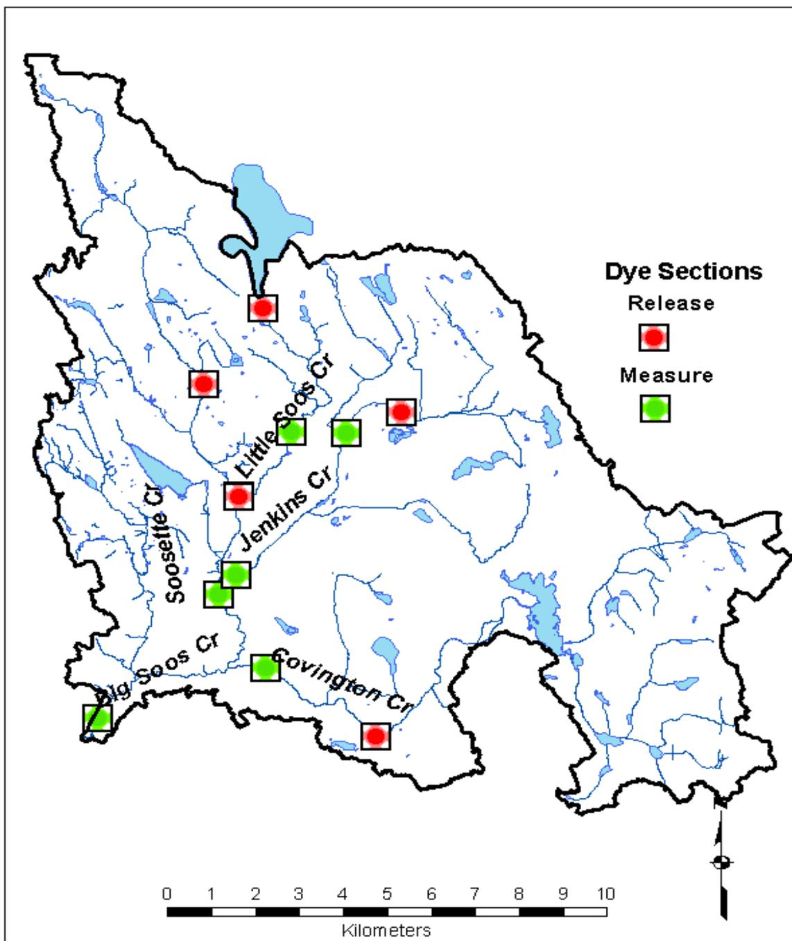
**FIGURE 8.** Release (red symbols) and measurement (green symbols) locations for time of travel study. Dye will be released at upstream locations and continuous measurement of dye concentrations taken until the peak of the plume has passed the downstream locations.
