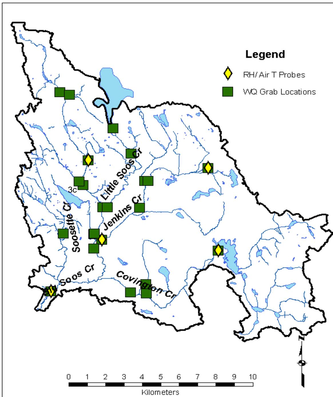
**FIGURE 7.** Twenty four water quality grab sampling locations, including continuous temperature data were collected during critical low flow periods in 2007 are mapped as green squares. Air temperature and relative humidity sensors are mapped as yellow diamonds.
