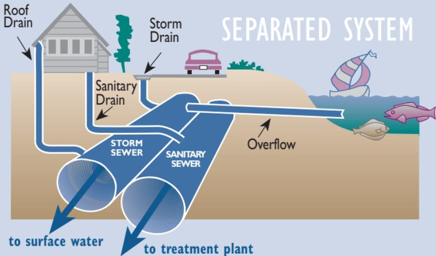
**FIGURE 5 – Combined and Separated Sewers**
