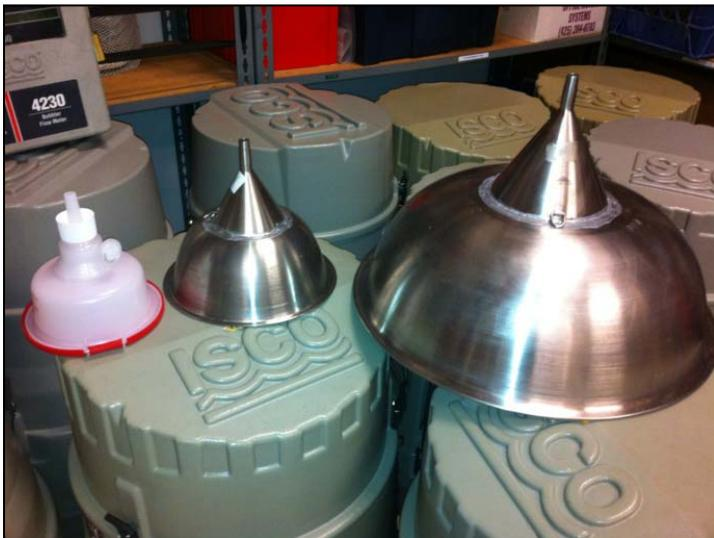
Large and small stainless steel funnels for organics and HDPE funnel for metals and mercury sample collection.
