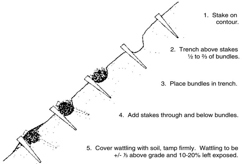
*NOTE: Installation starts at bottom of the bank and proceeds upslope, following steps 1 through 5.*
