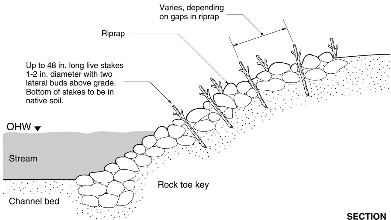
backfill or interstices. The basal ends should be cleanly cut at an angle for easy insertion into the soil; the top should be cut flat.
