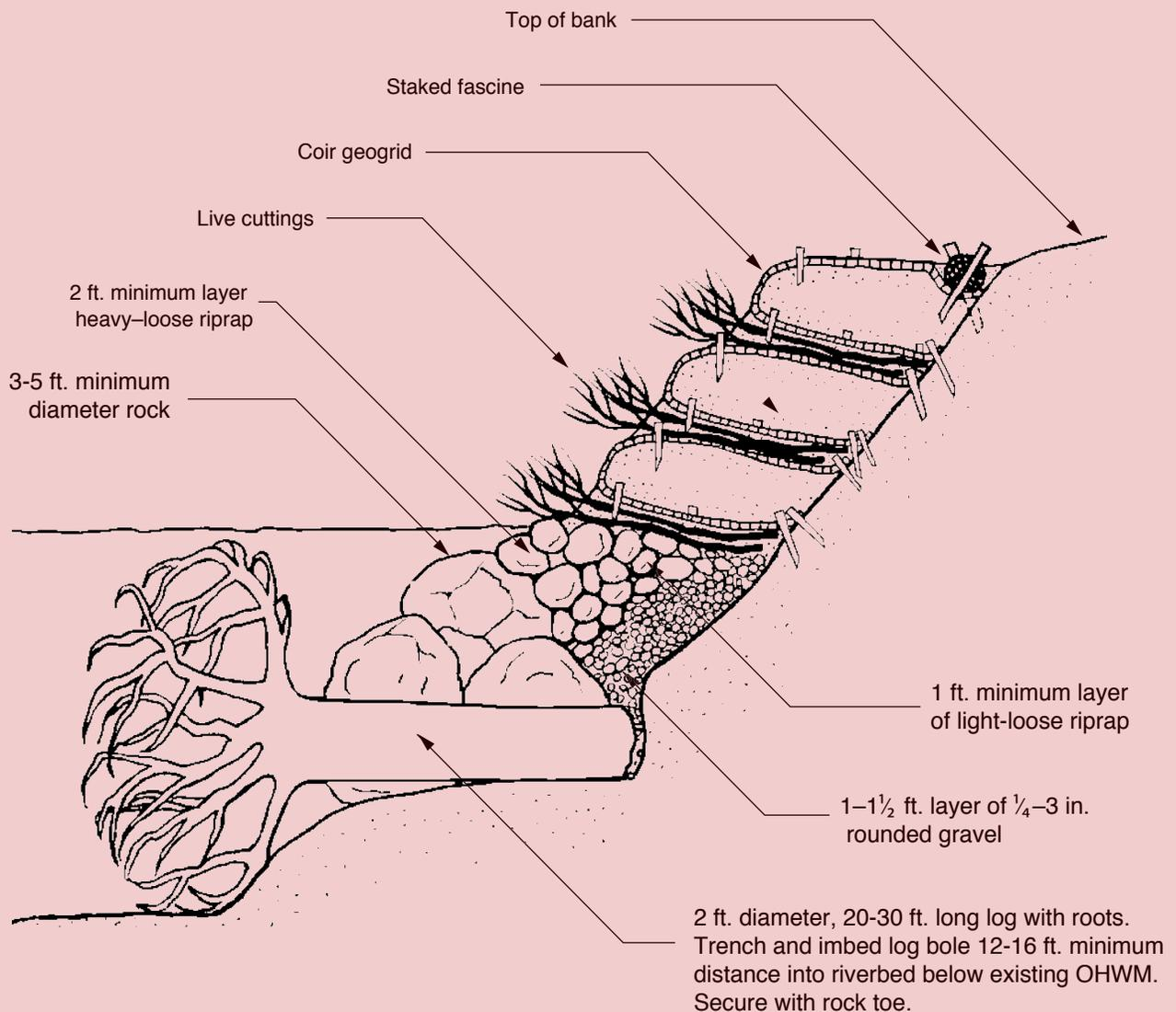
45 degree angle to the bankline and at 2 to 20 degrees downward towards the streambed. The entire log should be placed below OHW to keep it fully saturated at lower flows. It is recommended that layers of woody vegetative cuttings and topsoil be placed directly over the full dimension of the log and rock emplacement. The vegetation should be deeply rooting and tolerant of saturated soils.
