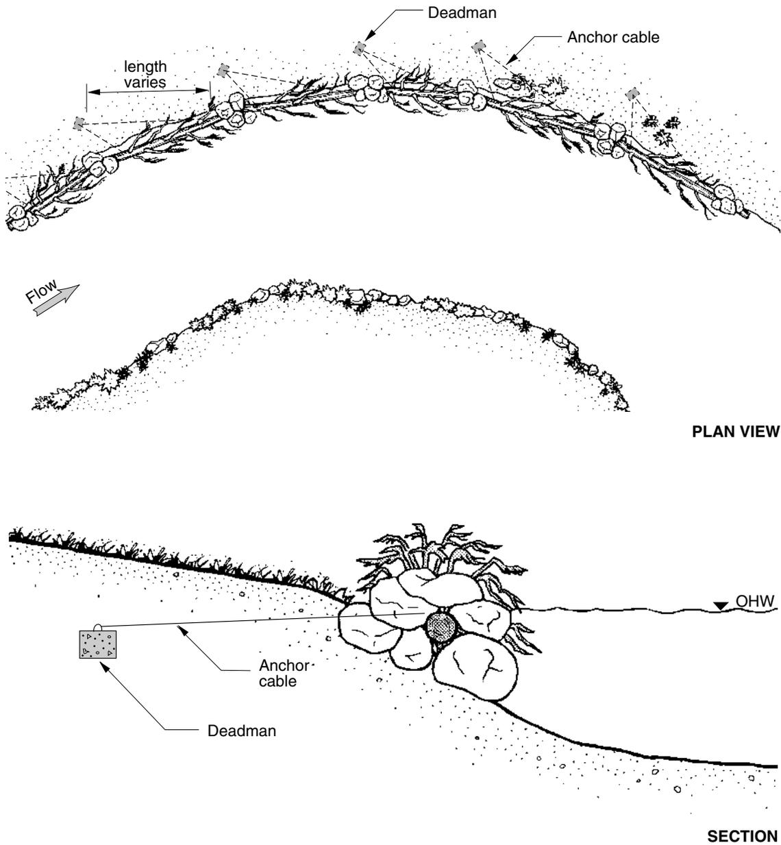
accomplished by drilling through the root and/or stump portion, passing a cable through the hole, and cementing each end of the cable to a large rock. A variation is to swage (i.e., crimp) a ferrule (i.e., bushing) around the cable; the free end is passed through a hole drilled through the center of the root and up through the center of the tree rings. The cable is then epoxied into a large boulder. If
