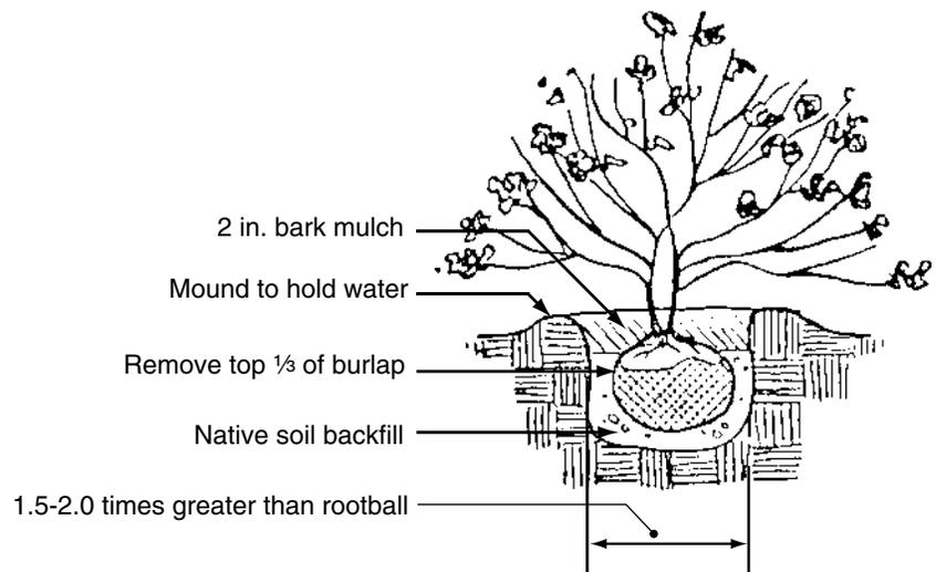
Figure 8.1c Installation of rooted stock—multi-stem tree.
